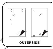
Explosion-Proof film helps to hold glass in place in the event of breakage. So as to prevent the glass shatter will hurt the user. Allowing the panel to be carefully removed by a professional at a later date.
