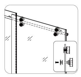
Adjust the fasteners on both Rollers (05) to ensure that the bottom edge of the Glass Door (07) will not touch the bottom of the Guide Block (11).
