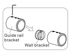
Loosen the screw on Guide Rail Bracket (02), pull out the wall bracket.
